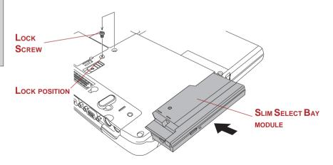
Figure 4-5 Inserting the Slim Select Bay HDD adaptor
